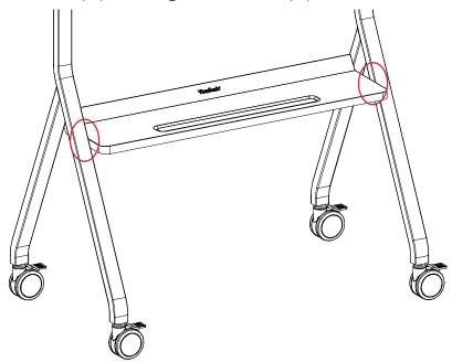
9. Secure the two Brackets (E) onto the display as shown below.
