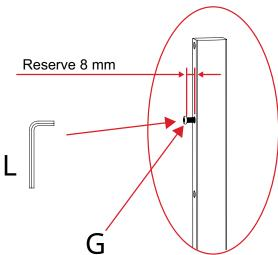
**5.** Hang the **Wall Plate** (**D**) onto the two halfway screwed **M8x16 Screws** (**G**). Once hung, fully tighten both **M8x16 Screws** (**G**).
