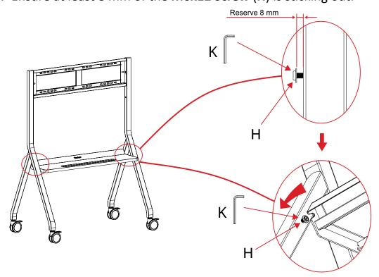
8. Place the Tray (C) onto the two exposed M6x12 Screws (H). Fully tighten the two M6x12 Screws (H). Using the remaining two M6x12 Screws (H), further secure the Tray (C) to the Left (A) and Right Columns (B).
