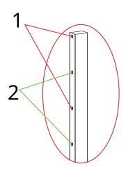
**4.** After choosing the appropriate combination, screw one **M8x16 Screw** (**G**) halfway into the middle mounting hole of the chosen combination into each **Column** (**A** & **B**).
