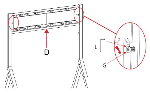
6. Screw in the remaining four M8x16 Screws (G) to fully secure the Wall Plate (D).
