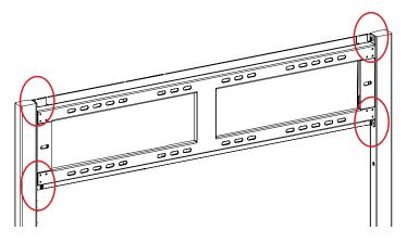
7. Screw one M6x12 Screw (H) halfway into each Column (A & B) as shown below.
