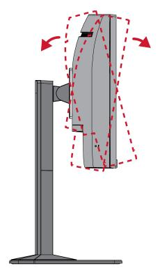
**NOTE:** When adjusting, support the stand firmly with one hand while tilting the monitor forwards or backwards with the other hand.
