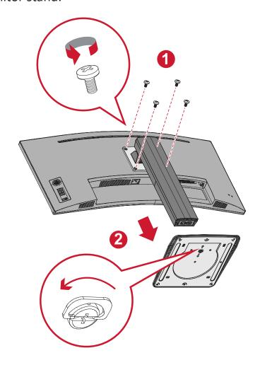
**4.** Attach the mounting bracket to the VESA mounting holes at the rear of the monitor. Then secure it with four (4) screws (M4 x 10 mm).
