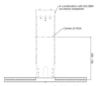
Can also be used above screen, by turning bracket upside down
