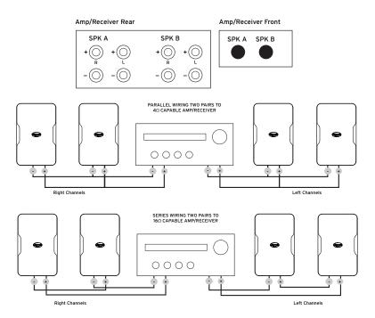
If your amp/receiver has separate connections for two speaker pairs, connect the two pairs of CP-6's to the two speaker terminal sets. Depending on your amp/receiver, either both pairs, or just one pair, will play at the same time.
