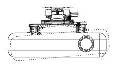
SWIVEL (YAW) 360° (when attached to extension column) +/- 15° (when flush mounted)
