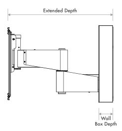
Height: 20.76" [52.7 cm] Width: 32.76" [83.2 cm] Total Depth: 4.44" [11.3 cm] Ext. Depth: 28.59" [72.6 cm] Wall Box Depth: 3.85" [9.75 cm]
