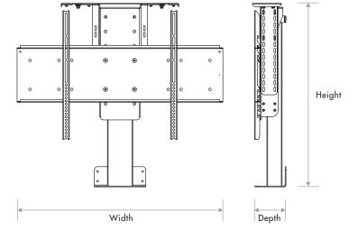
Height: 72.4 cm Min / 102.9 cm Max Adjustable in .6 cm increments
