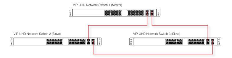
Whilst it is not necessary to have a link between switches 2 and 3 as shown above, this will act as a back-up loop ensuring that should one of the uplinks fail, then the multicast streams can take an alternative route to provide the streams to their intended destination regardless of where the VIP-UHD transmitter and receivers are located.
