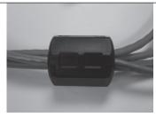
Ferrite ring closed - with cables
