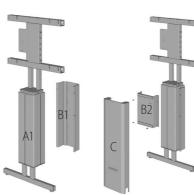
4. Place the lift (A1) in the wall mount (B1) and lock this with the small front plate (B2). Fasten the screws B2 on B1. Put the front plate (C) in position and fasten it with the Velcro tape.
