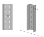
3. Drill a minimum of four holes in the constructive wall and secure the wall mount plate (B1).
