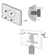
6. Place the 4 VESA screws in the back plate of the display. Place the display on the H-bracket (A2) and tighten the VESA screws.
