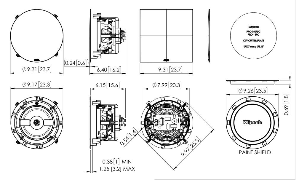
MODEL: PRO-16RC DATE: 2018-02-02 DIM: SHEET: 1 OF 1 SCALE: 1:5
