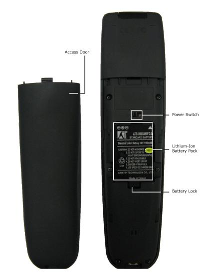
Follow the steps below to install/access the rechargeable Lithium-Ion battery.
