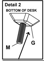
NOTE: Avoid jamming both slope nuts (G) together, doing so may make it difficult to remove slope nut used for tightening.
