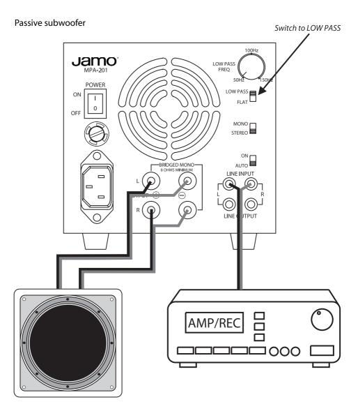
When "Low pass" is selected, you can adjust the low pass frequency between 50 - 150 Hz. This makes it possible to make the subwoofer match your front speakers.
