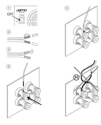
**Note:** Make sure that the stripped + and - wires do not touch each other, as a short-circuit could damage the Jamo MPA-201's output section.
