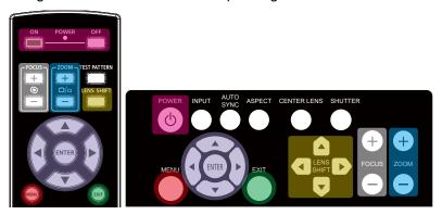
Press the Menu button on the projector control panel or remote control to open the OSD. There are five folders (Input, Picture, Alignment, Control, Service) on the menu. Press the cursor ◀ or ▶ buttons to move through secondary menus.
