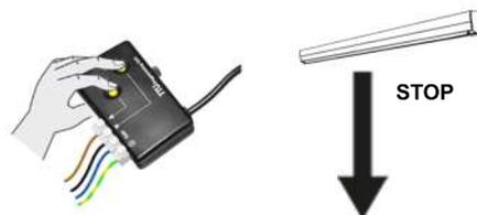
7. Push the down button again. Make the screen go down till the approximate desired down limit position (when you push the down button, the motor starts slowly, makes a short STOP and then it becomes faster);
