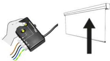
5. Push the up button again. Make the screen go up till the upper stop position. Once there, the motor will stop automatically; Do not leave the button, but keep the button pushed.
