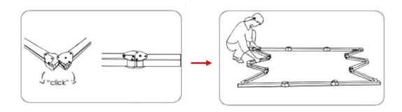
**Note:** When unfolding the frame and legs, be sure the latches on the hinges "click" into place. Please also make sure all 4 corners of the frame are at a 90° angle and the hinged support bar is straight and not bent.
