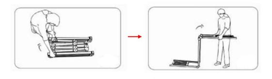
2. Next, unfold the frame until the latch on the hinge "clicks" into place. Repeat the procedure for the shorter sections, as shown below.
