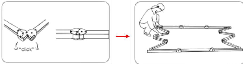
**Note:** When unfolding the frame and legs, be sure the latches on the hinges "click" into place. Please also make sure all 4 corners of the frame are at a 90° angle and the hinged support bar is straight and not bent.
