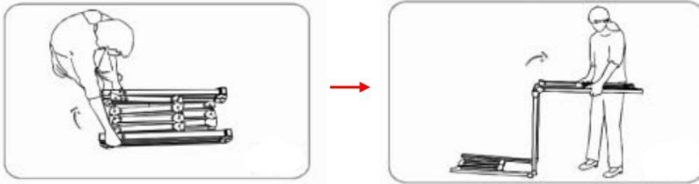
2. Next, unfold the frame until the latch on the hinge “clicks” into place. Repeat the procedure for the shorter sections, as shown below.
