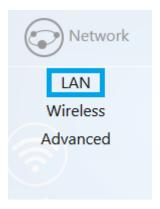
Hover over the **Network** icon and click **LAN**. This page displays the LAN settings for the WK-1x. To configure the IP address of your WK-1x, you can configure the WK-1x with a static IP address or obtain an IP address automatically by using a DHCP client.
